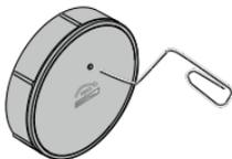
Press **P button** on the **new** transmitter for 6 seconds.
