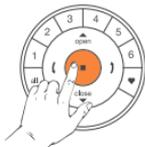
Press **Stop button** on the known transmitter for 6 seconds or wait for 20 seconds
