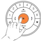
Press **Stop button** on the known transmitter for 6 seconds.
