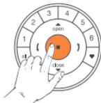
Press **Stop button** for 6 seconds → Button lighting on the transmitter stops flashing.
