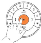
Press **Stop button** for 6 seconds → Button lighting on the transmitter flashes. Teach-in readiness established.
