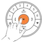
Press **Stop button** for 6 seconds → Button lighting on the transmitter flashes.
